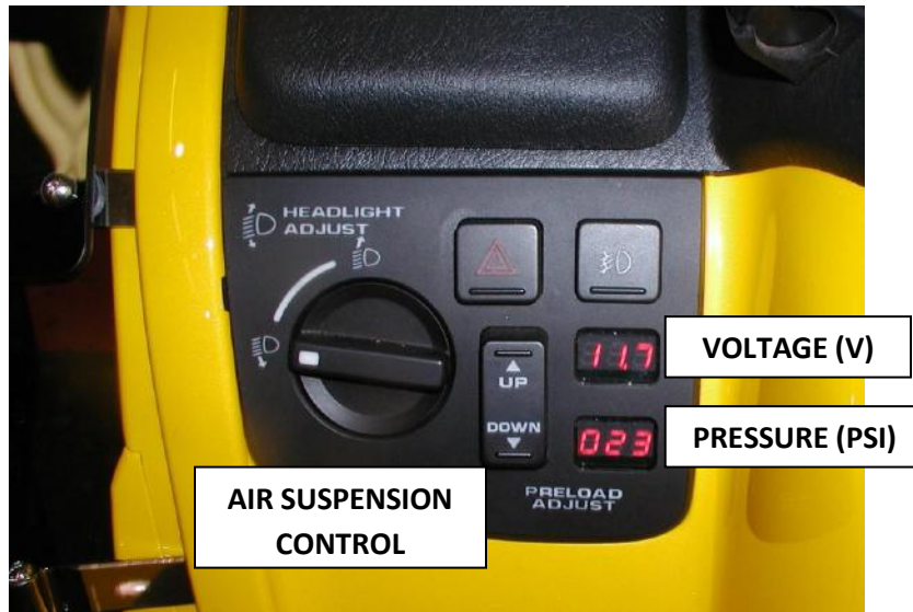
Figure 2: Air suspension control panel
