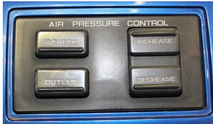
Figure 3: Air pressure control panel
