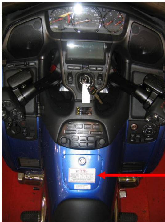
Figure 4: Location of the air suspension pressure recommendation sticker
