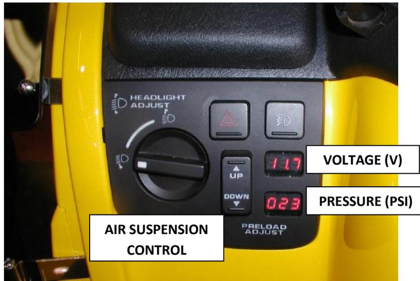
**Figure 2: Air suspension control panel**
