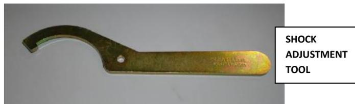
To adjust the shock, hook the end of the shock adjustment tool into the bottom portion of the shock and rotate the collar clockwise to raise the trailer to the desired setting. It is important that both shocks be set to the same setting. In order to prevent physical injury or vehicle damage, only remove one tire at a time with the opposite tire chalked and the vehicle on level ground.
